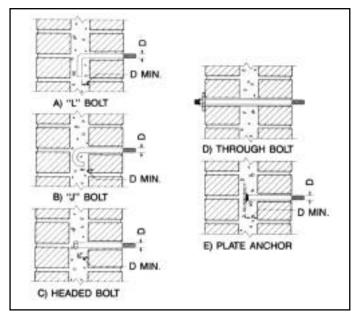
Conventional Anchors in Grouted Collar Joints FIG. 12
