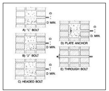
Conventional Anchors in Multi-Wythe Brick Masonry FIG. 13
