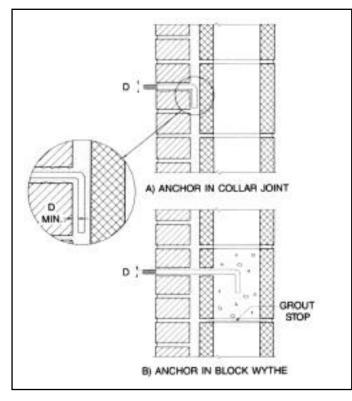
Conventional Anchors in Composite Brick/Block Masonry FIG. 17
