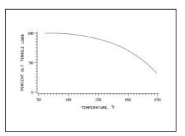
Effect of Temperature on Ultimate Tensile Capacity FIG. 11
