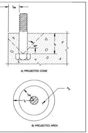
Reduced Masonry Tension Cone FIG. 20
