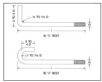
"L" and "J" Bent Bar Anchors FIG. 2
